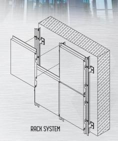
A light, ventilated façade system consisting of composite panels and mounting profiles and accessories.
